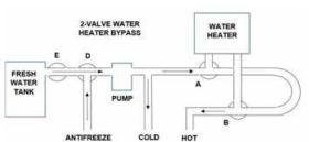
NORMAL - VALVE HANDLES A & B POINT TOWARD THE WATER HEATER.
